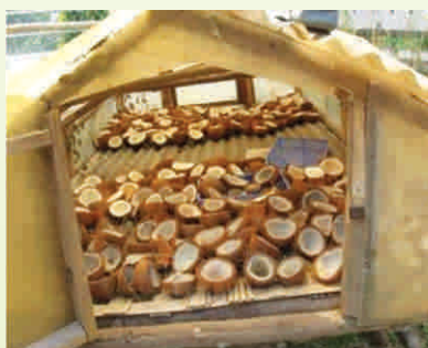
Low cost solar dryer
